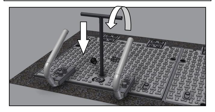
Whilst the Slam Latch mechanism is still levered open, use the lifting handles to lift the cover. After the cover has opened and has cleared the frame, the Tommy bar can be removed.
